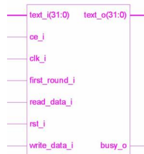
Fig. 5 SHA block structure
